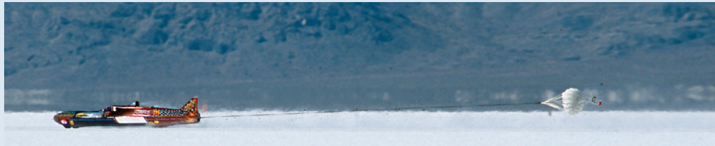
Above: Vesco heard the tire explode just as he finished the 458MPH record run. Look closely and you can see tire fragments trailing behind the car, a couple of big chunks are just above the drogue chute behind the canopy. This was truly a "run flat" tire. Below: The late Don Vesco, multiple World Land Speed Record holder in 2001.
